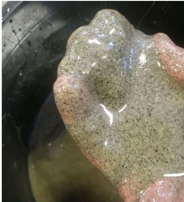
Figure 3.3 – Shows the viscosity being measured. The time shown translates to 180sec/L viscosity and a density of 1922kg/m 3 .
