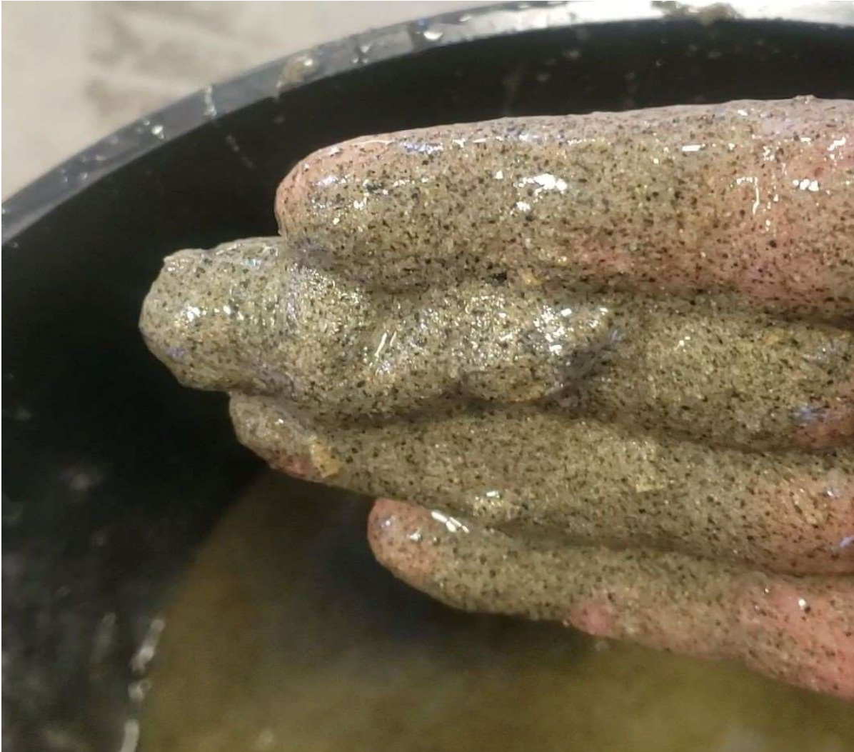
Figure 3.5 - Illustrating high concentration of sand. The sand content on this particular test was 78% sand in solution.
