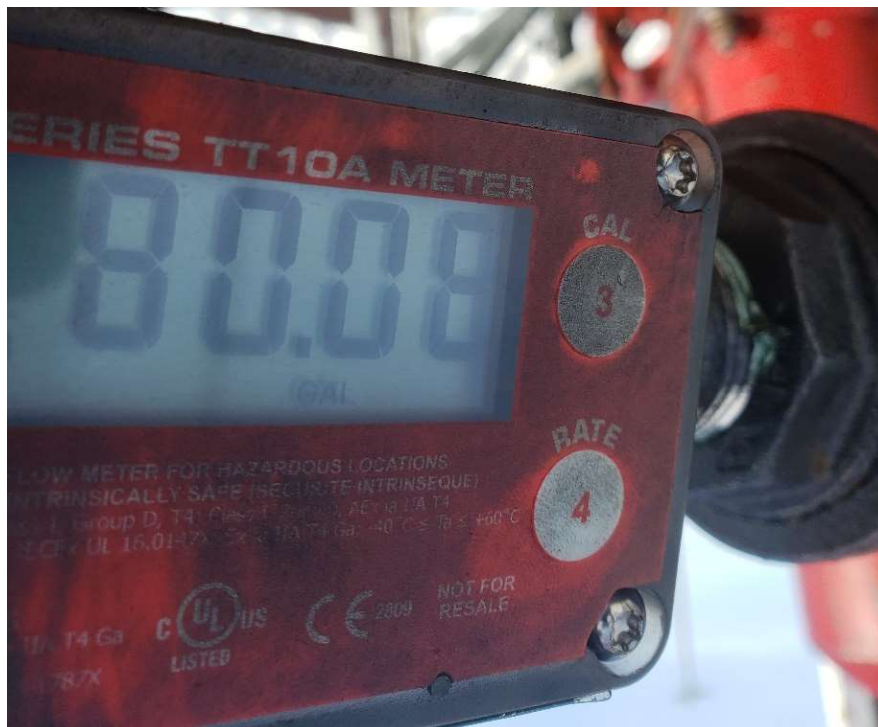
Figure 3.5 - Test # 2 Digital flow meter read out after 20 strokes @ 5 strokes /min with 16' stroke.
