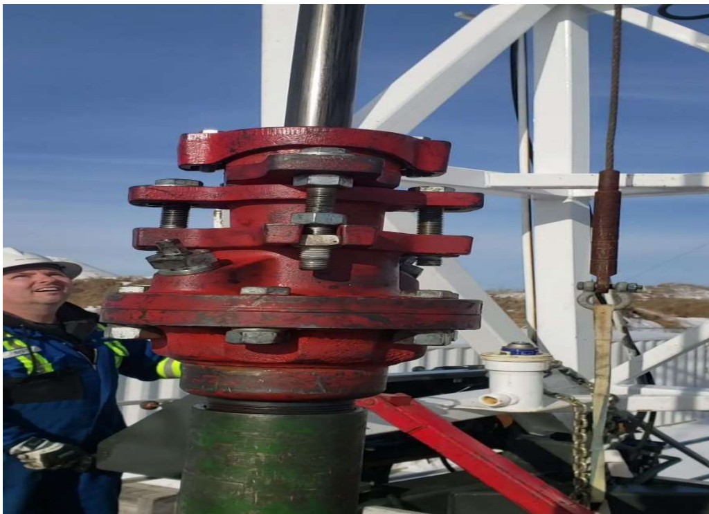
Figure 2.3 – Stuffing box installed on tubing with 1 ½ polish rod.
