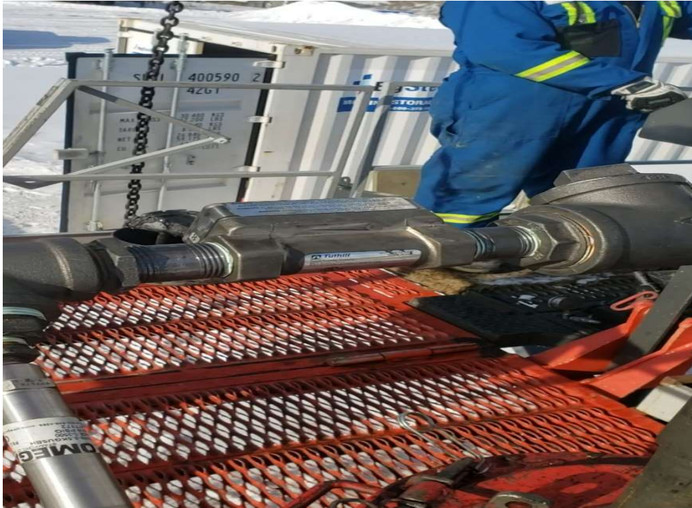
Figure 2.2 – Digital flow meter and pressure transducer installed on flow line.
