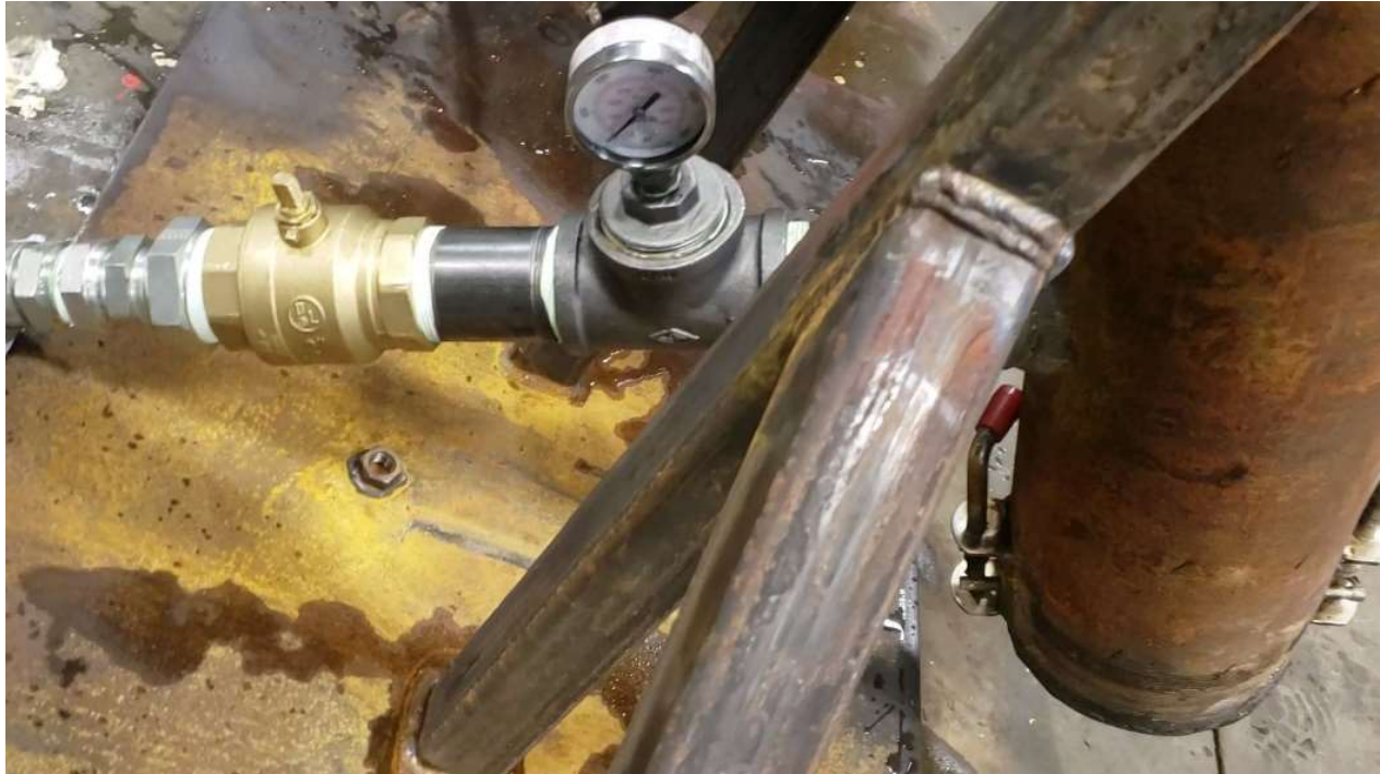
Figure 2.3 – Return line with valve and pressure gauge.
