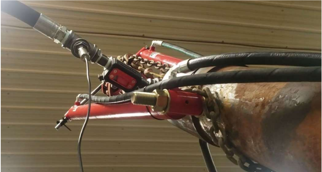
Figure 2.2 – Flow rite flow meter and Omega Pressure Transducer installed on flow line.
