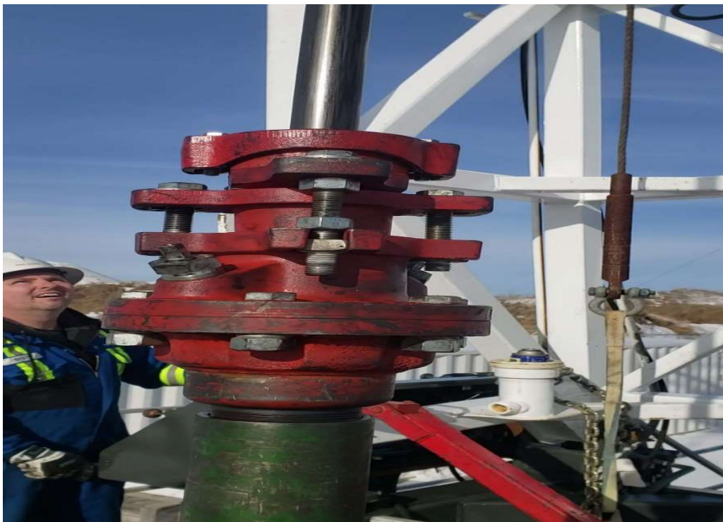
Figure 2.3 – Stuffing box installed on tubing with 1 ½ polished rod.
