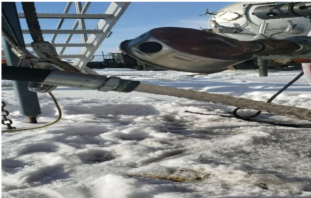
Figure 3.3 – Bleeding air out of the lines prior to circulating a closed loop. Hose size is 1 1/2".
